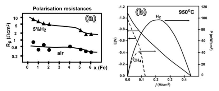
Fig. 3. (a) Dependence of Polarisation Resistances ( $R_p$ ) with the Fe content, at 900°C, in the La<sub>4</sub>Sr<sub>8</sub>Ti<sub>12x</sub>Fe<sub>x</sub>O<sub>38-8</sub> system (29). (b) Fuel Cell test performances using LSTF symmetrical electrode, at 950°C, with different gases.
