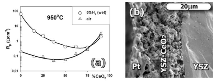
Fig. 4. (a) Dependence of the Polarisations Resistances ( $R_p$ ) with the CeO<sub>2</sub> content, at 950°C, for the cermets Pt-YSZ-CeO<sub>2</sub>, under air and humidified 5% H<sub>2</sub>. (b) SEM image of a cross-section of a Pt-YSZ-CeO<sub>2</sub> based symmetrical SOFC (30).
