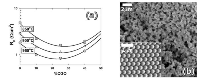
Fig. 2. (a) Dependence of Polarisation Resistances ( $R_p$ ) with the CGO content in (LSCM-YSZ-CGO)-based symmetrical cells, at different temperatures (3). (b) SEM image of the microstructure of LSCM-YSZ symmetrical electrode prepared using PMMA microspheres (15).
